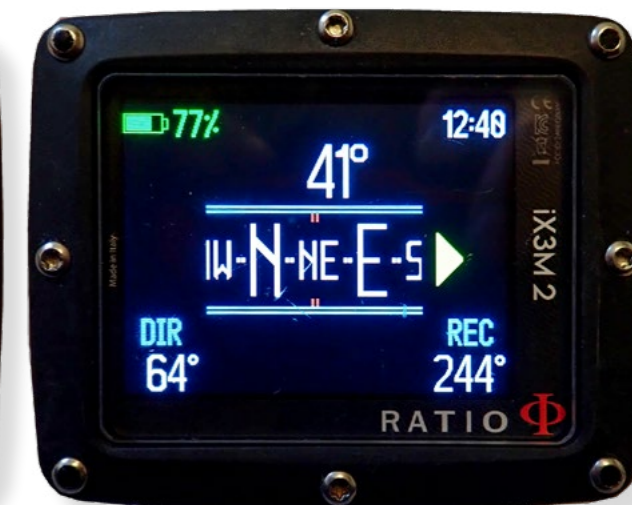
The compass on the Ratio iX3M 2 dive computer shows direction on and off course.
