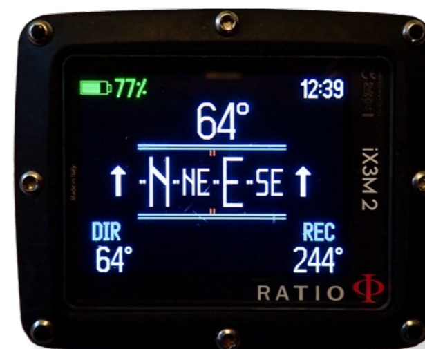
The compass on the Ratio iX3M 2 dive computer shows direction on and off course.
