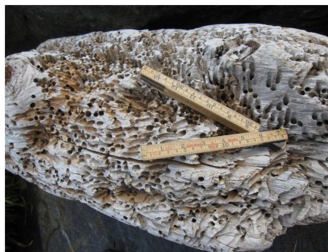
Shipworm holes (above and right) in a salvaged piece of wood. The Teredo navalis species of shipworm usually grows up to 30cm long, but has been known to reach up to 60cm in length and 1-2cm in diameter.
