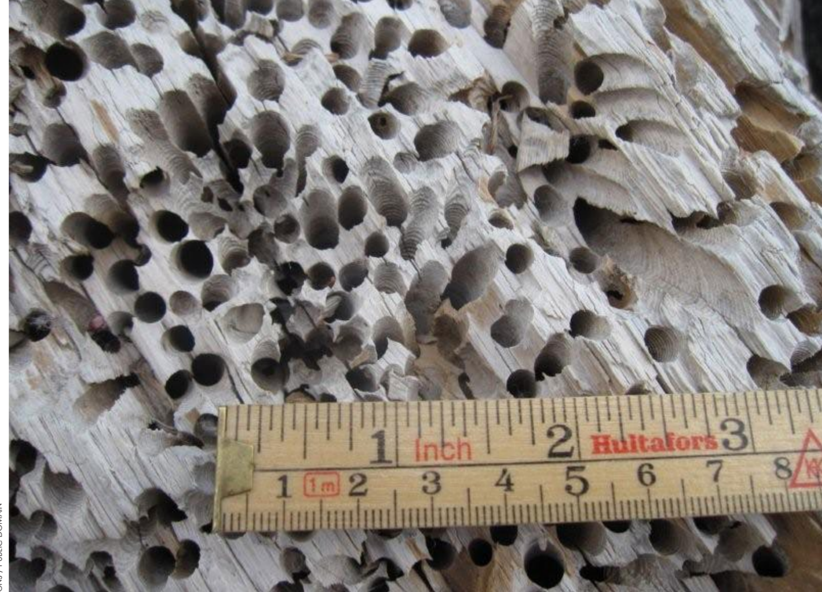
Shipworm holes (above and right) in a salvaged piece of wood. The Teredo navalis species of shipworm usually grows up to 30cm long, but has been known to reach up to 60cm in length and 1-2cm in diameter.
