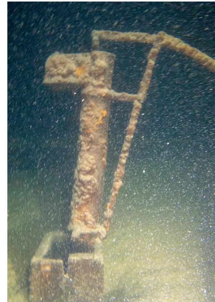
A hand pump used to remove bilge water (above); Diagram of the first wreck site (left)
