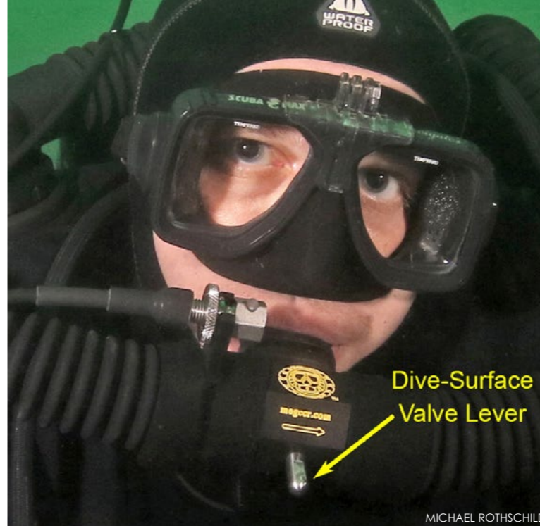
Figure 2: Dive-surface valve (DSV) vs. bailout valve (BOV)
