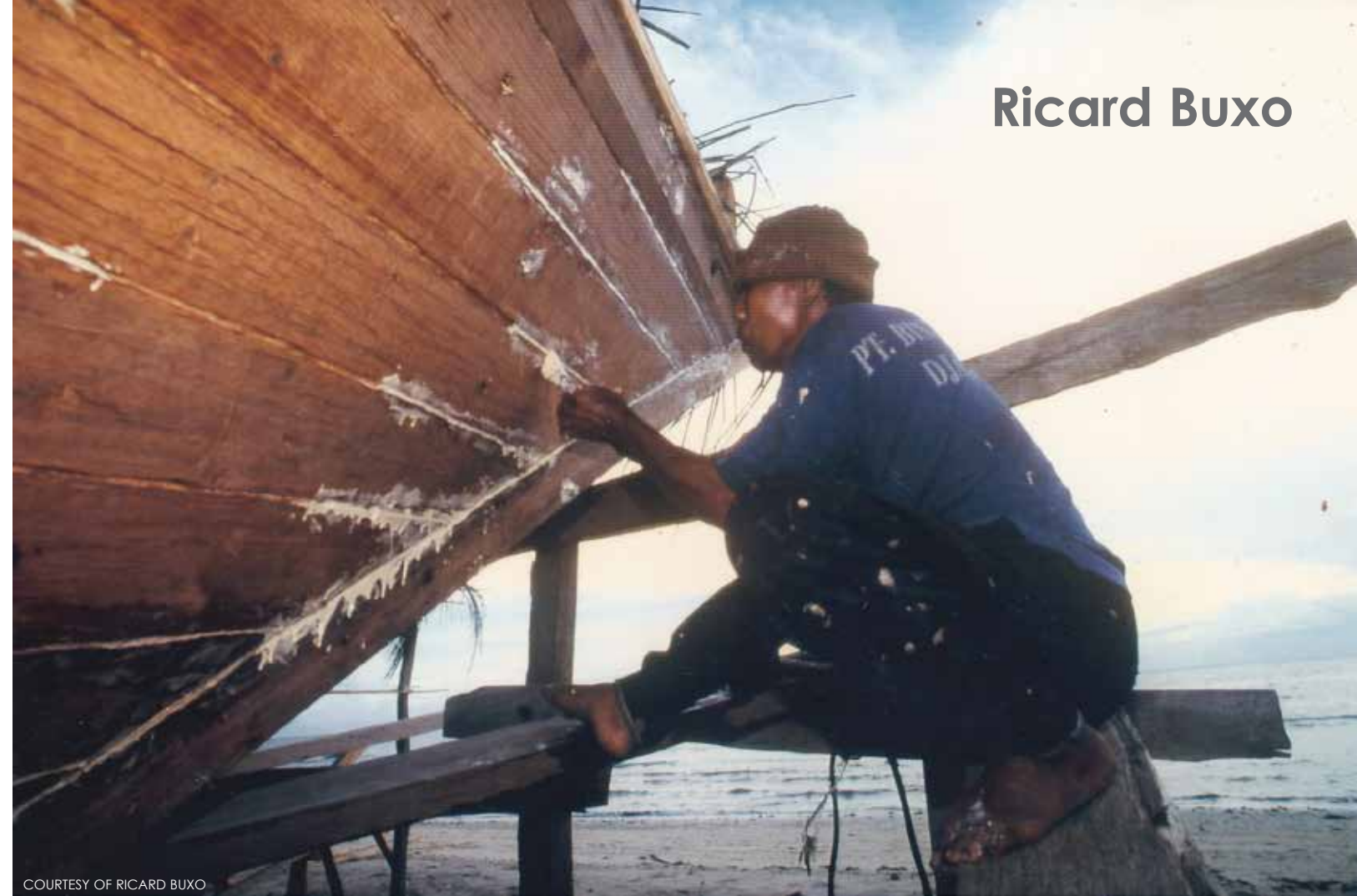
Laying the main deck of the Ondina (top left); Sealing the hull (top right); The pinisi boat under construction at Tanah Beru (right); The lounge and dining area under construction (left)
