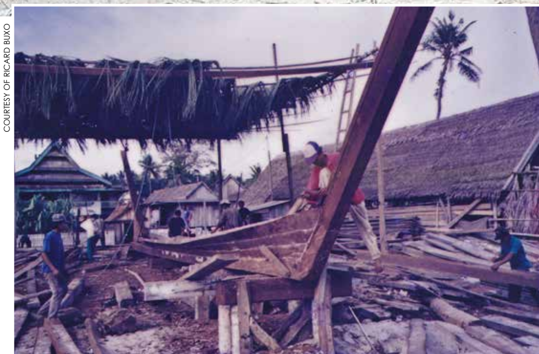
The hull of the Ondina taking shape (left)
