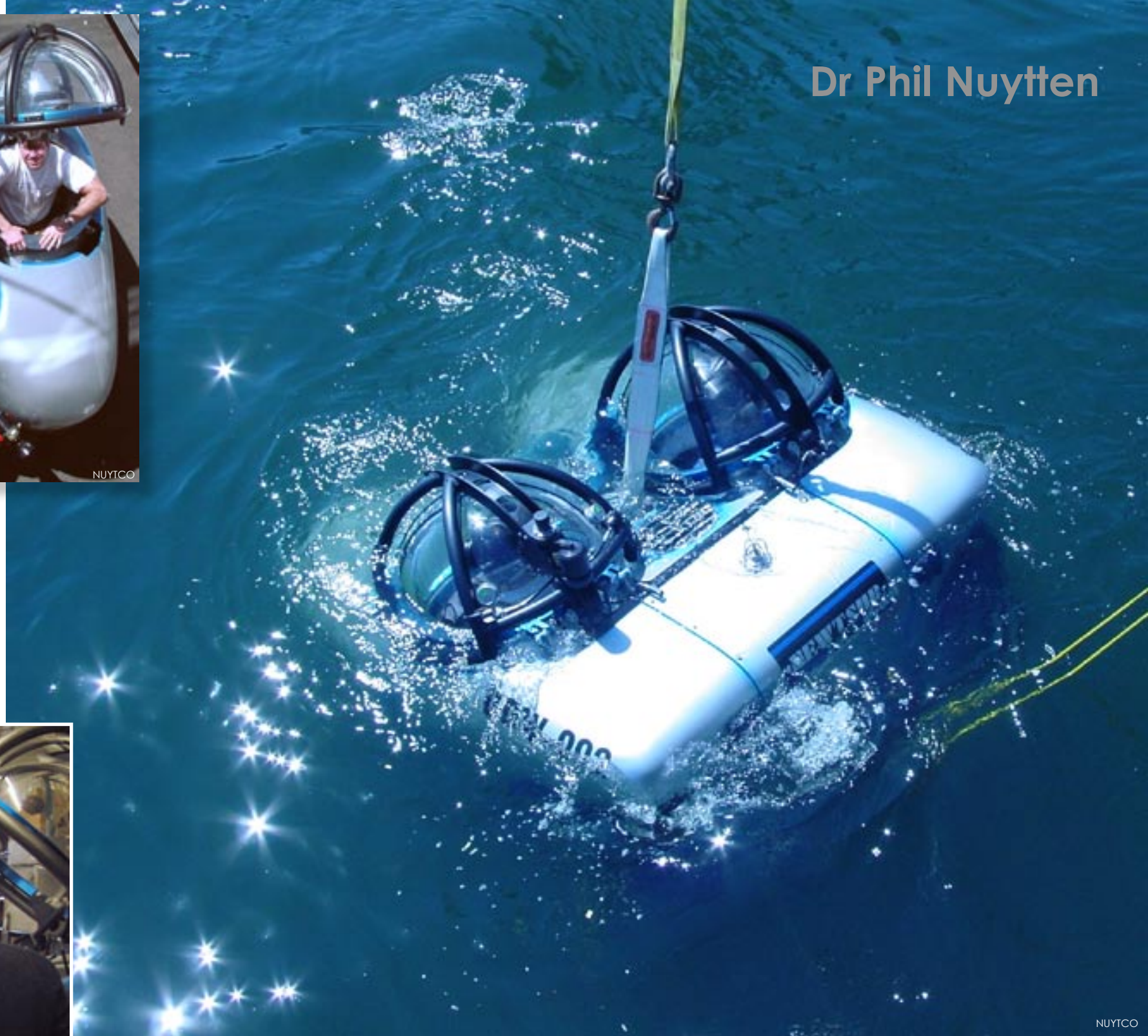
The two-person Dual DeepWorker NewtSub submersible is lowered into the sea
