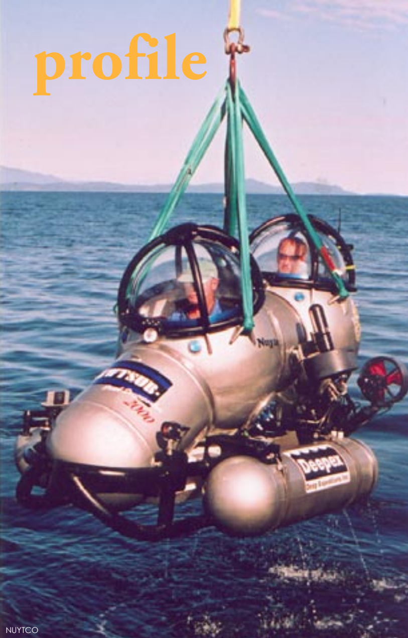
LEFT: The two-person submersible, Dual DeepWorker NewtSub, allows for a pilot and an observer
