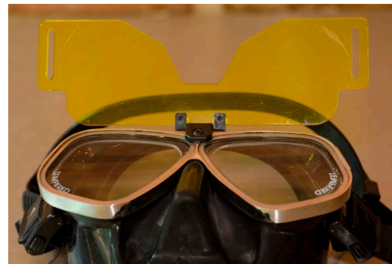
Dive 2000 designed swing filter visor that hinges from the mask frame and semi locks at three positions
