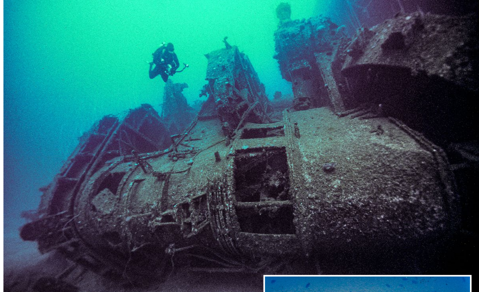
The 16-inch guns (left) on the wreck of the Japanese battleship Nagato , at 180ft, and the bridge (above), which broke off when the ship sank upside-down at Bikini Atoll
