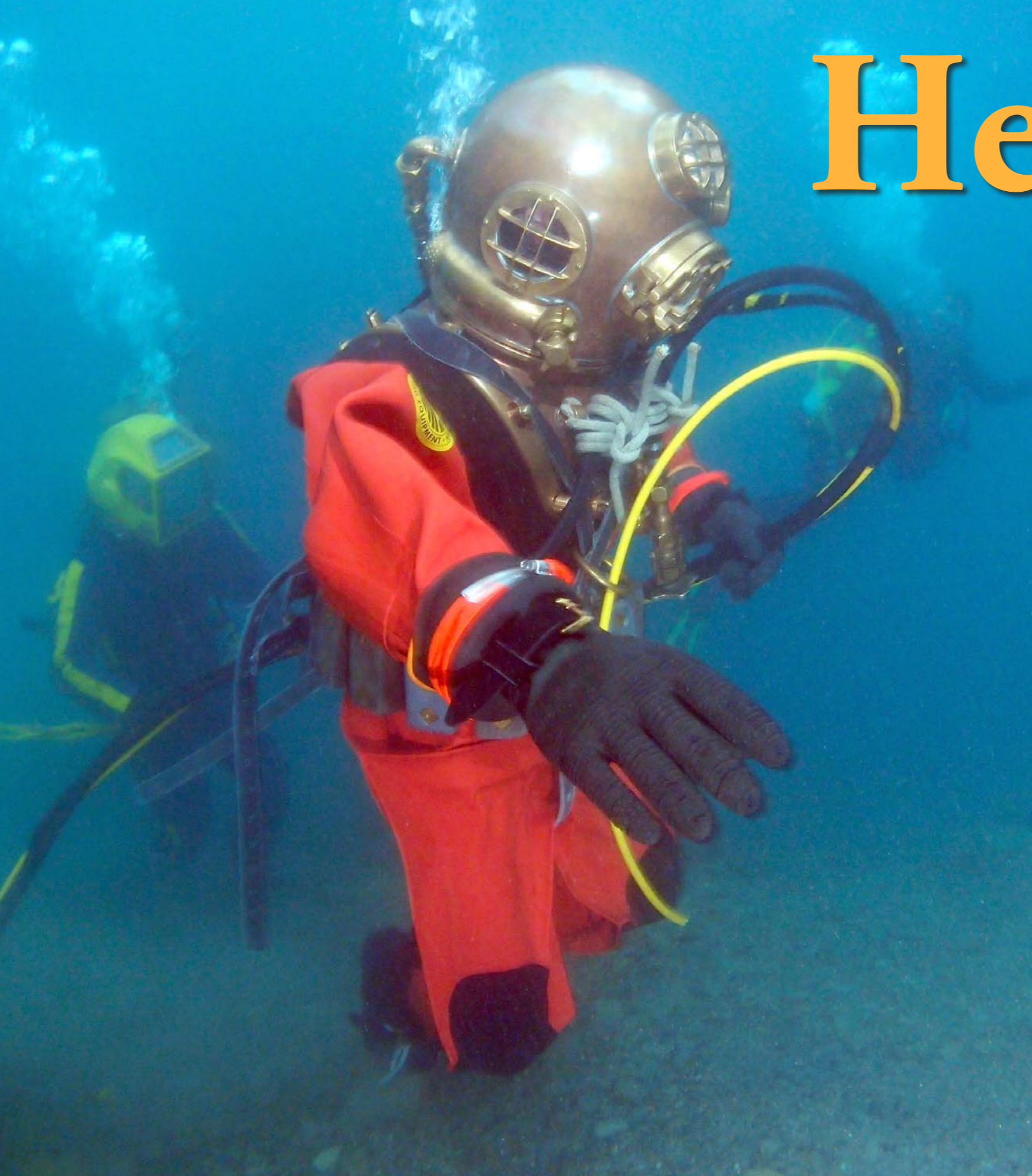
Diver in Mark V helmet and diver in background in Mark XII helmet
