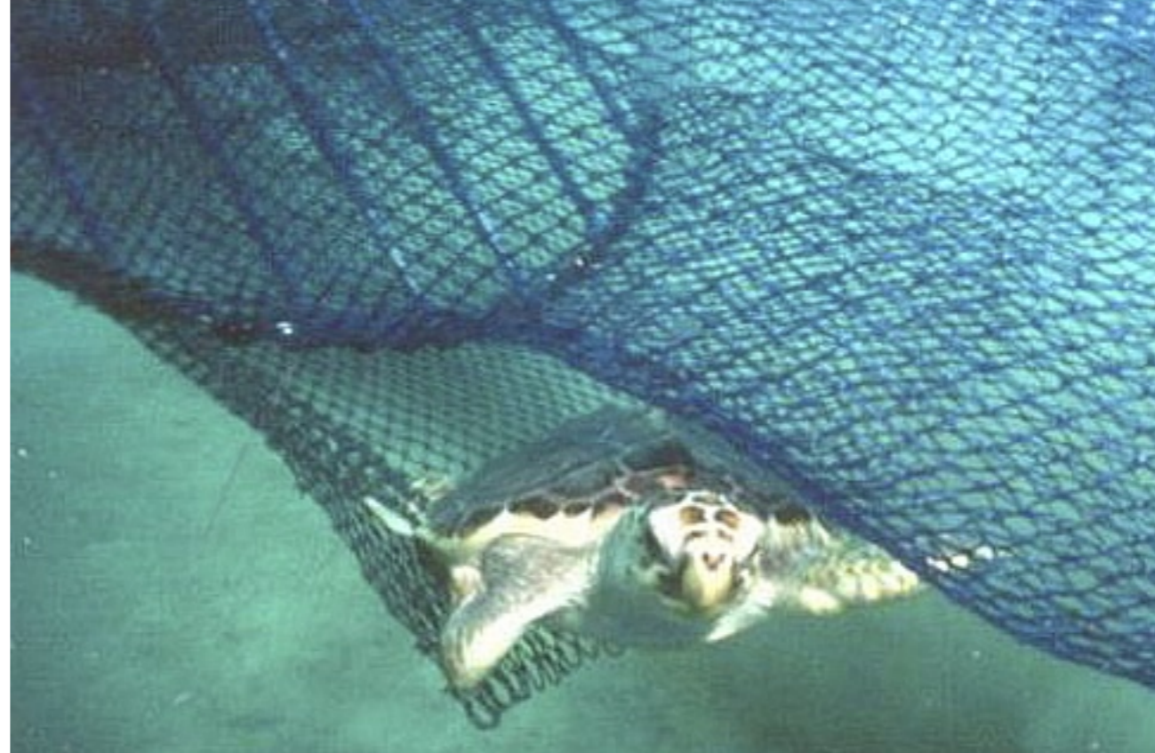
A "Turtle Excluder Device" is a grid of bars with an opening either at the top or the bottom of the trawl net. The grid is fitted into the neck of a shrimp trawl. Small animals such as shrimp pass through the bars and are caught in the bag end of the trawl. When larger animals, such as marine turtles and sharks are captured in the trawl they strike the grid bars and are ejected through the opening
