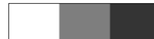
The standard grey card has a 18% reflectancy (middle). This is the golden standard against which light meters are calibrated and white balanced measured
