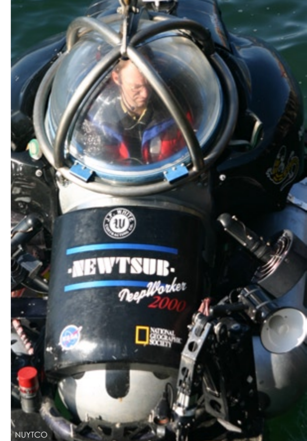
Close-up of the one-person DeepWorker used by National Geographic
