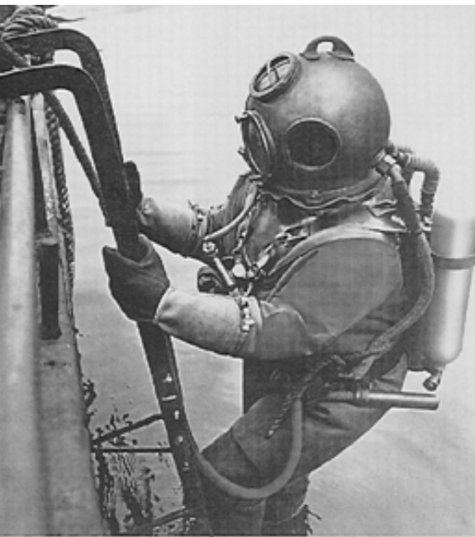
No, rebreathers are not new. In this 1912-footage we see Dräger's helmet diving rebreather in use. Photo: Dräger's archive.
