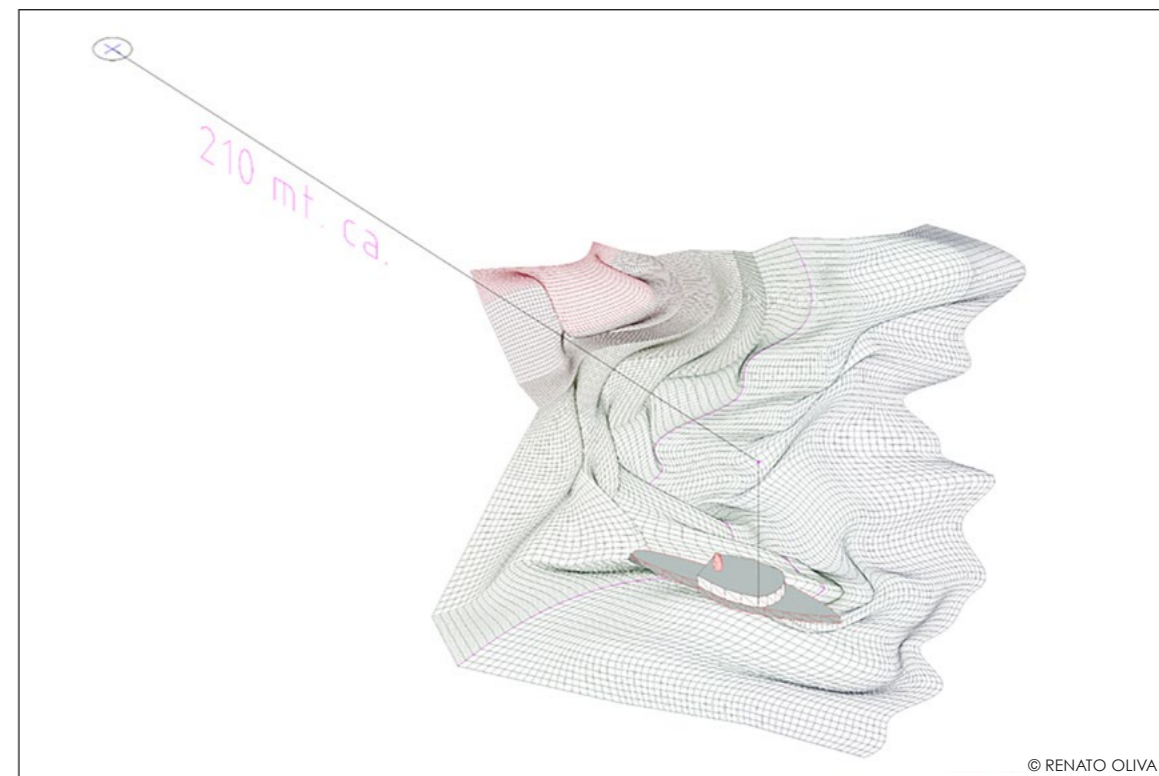
This 3D model shows the wreck of the Plinio III on the bottom of Lake Mezzola and its distance from the shore (in metres). Drawing by Renato Oliva
