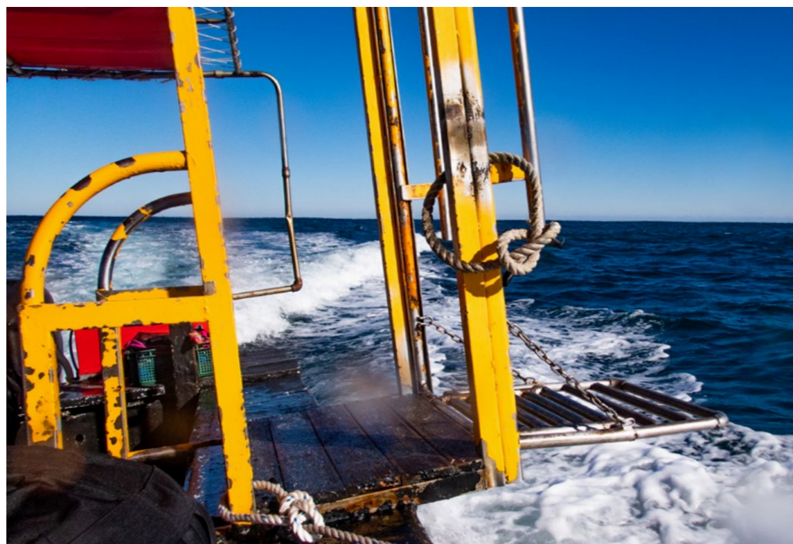
An elevator platform is commonly used to lift divers and their gear from the tag line to the dive boat.
