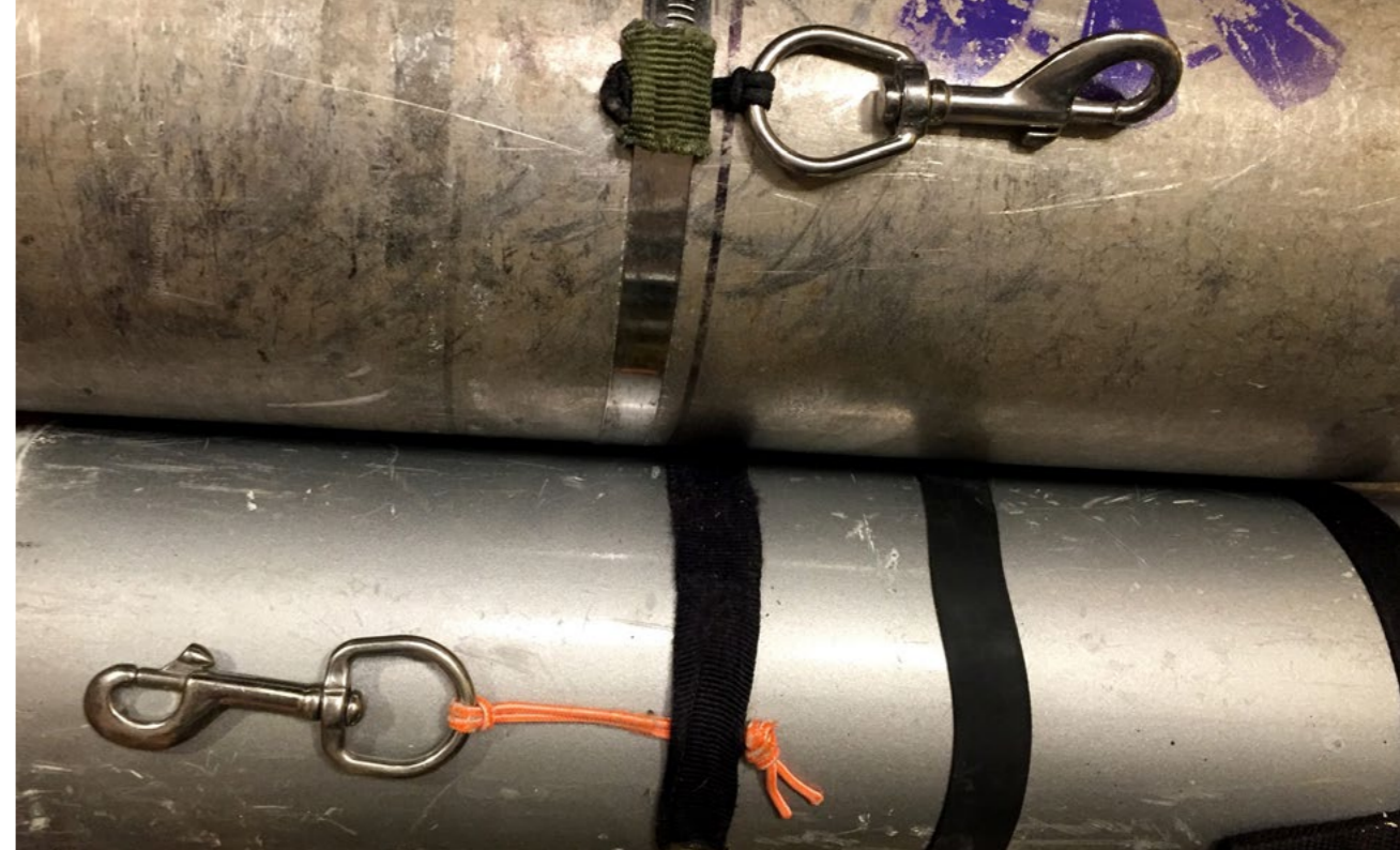
Photo 5. Leash lengths (note the longer leash usually used for steel tanks and the nearly non-existent length for aluminum tanks)
