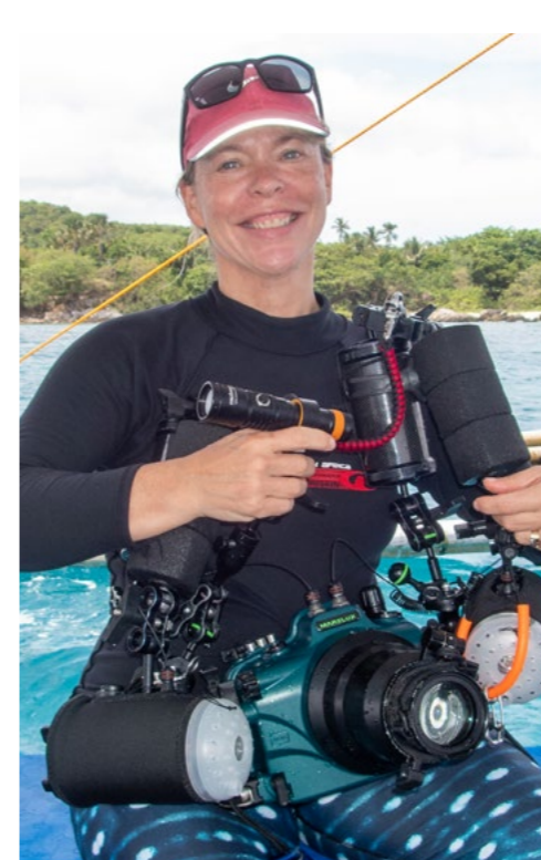
Kate Jonker with her macro underwater setup (above): Canon R5 camera with 100mm macro lens in Marelux housing and two SUPE D-Pro strobes, plus Orcatorch D710V for spotting and focus light and Fantasea UCL-09F diopter (+12.5); Pink noble coral at Steenbras Deep, Gordon's Bay. Equipment: Canon R5 camera with Canon 8-15mm circular fish-eye lens, Marelux housing, and two SUPE D-Pro strobes. Settings: f/7.1, 1/125, ISO 500
