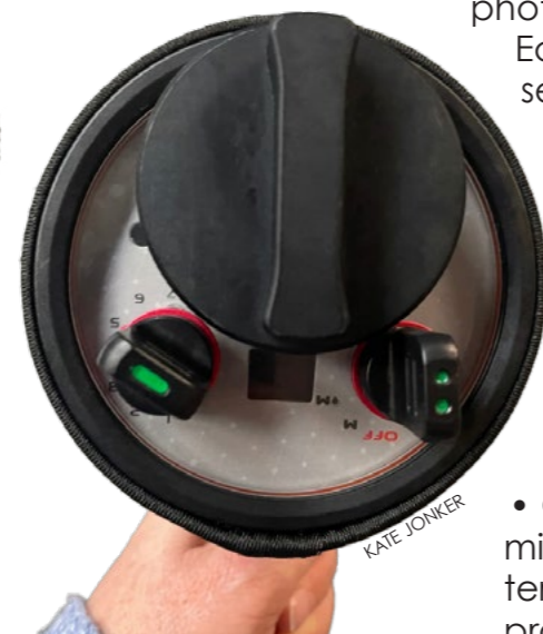
Front view of SUPE D-Pro strobe, showing circular flash tube and central focus light, and rear view, showing On-Off knob (on the right) and Power knob (on the left).
