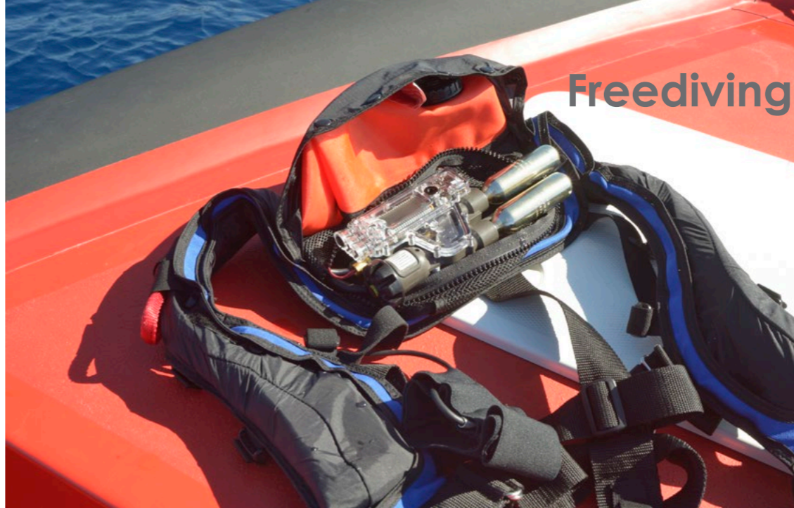
Freediver Recovery Vest (FRV) electronics and two 38-gram CO 2 cartridges, which provide sufficient lift from depths of up to 45 meters
