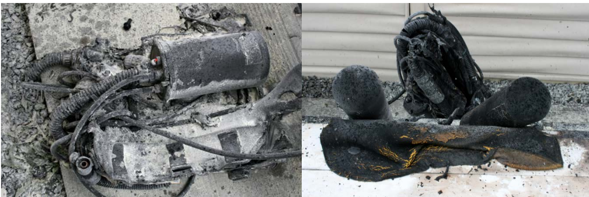
Figure 2. Results of small, localized rebreather fire.
