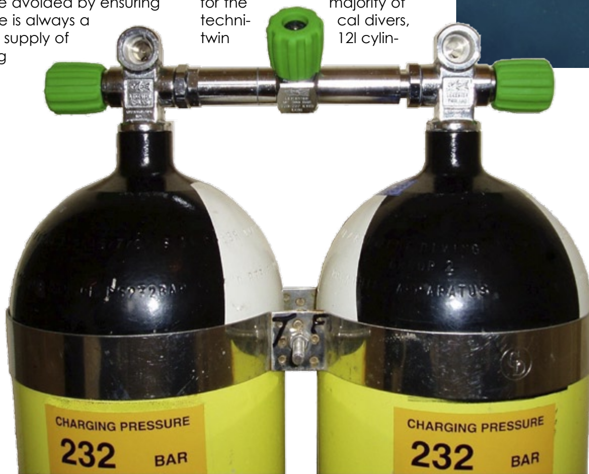
In twinsets, the two cylinders are often connected at the valves by means of a manifold
