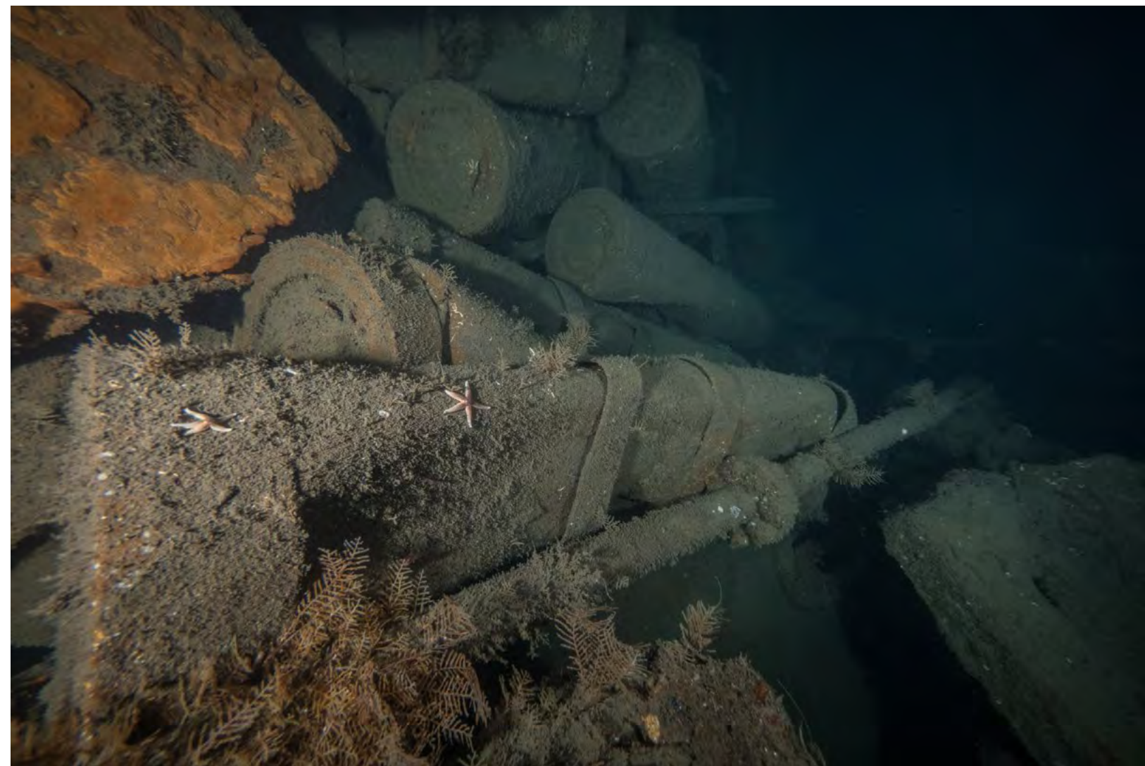
Clarkson cases on HMS Queen Mary . The propellant for the guns was kept in these cases. Poor handling and storage of them was one of the major contributing factors to the way the British battlecruisers blew up.
