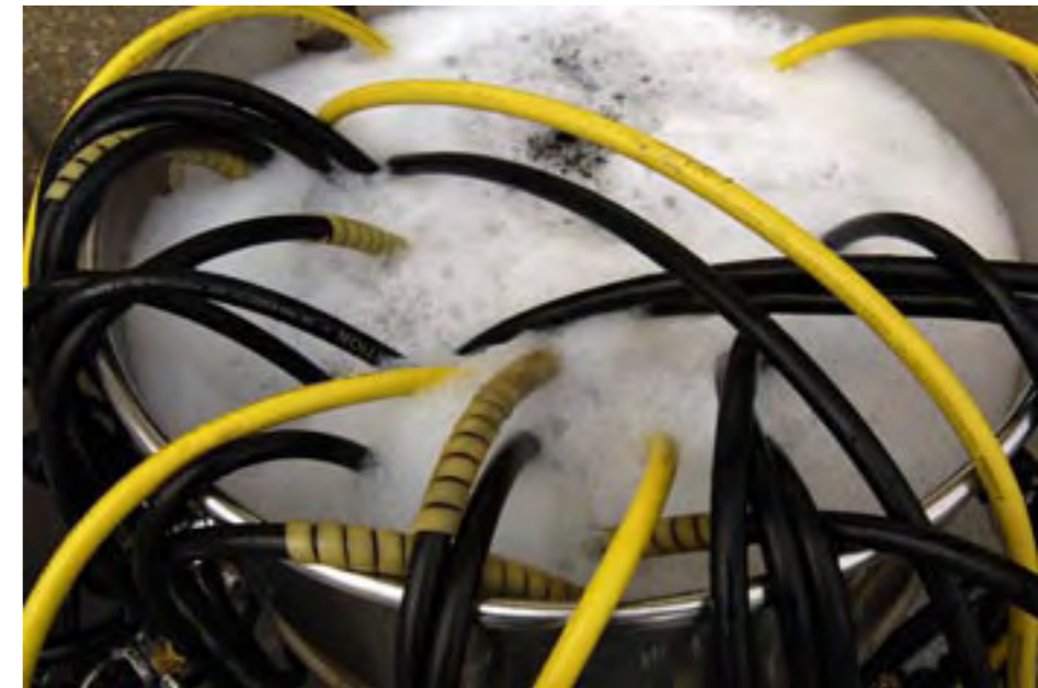
A bath of cleaning solution is used to sterilize scuba regulators used by diving students at the Naval Diving and Salvage Training Center here. The regulators are cleaned after each diving exercise at the center
