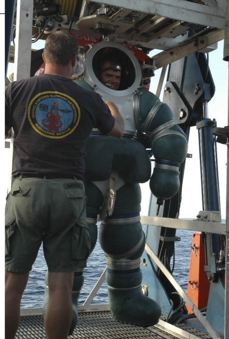
Chief Navy Diver Daniel Jackson completes a successful certification dive of the Atmospheric Diving System (ADS) aboard the special mission charter ship M/V Kellie Chouest
