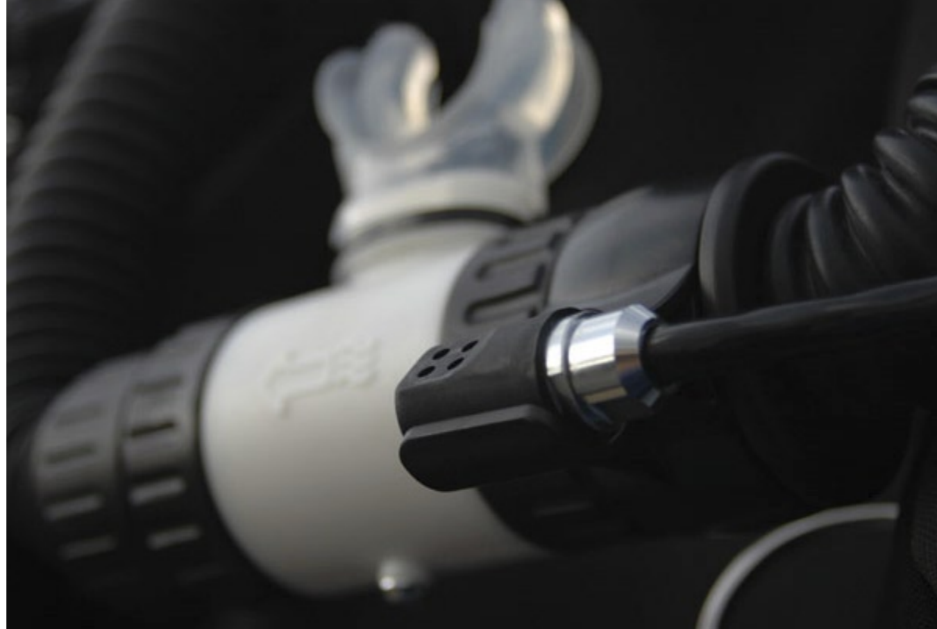
Close-up of the Head-Up display unit (HUD) on Inspiration/Evolution mouthpiece
