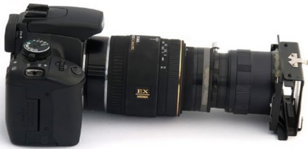
Figure 1. DSLR camera with macro lens and slide duplicator
