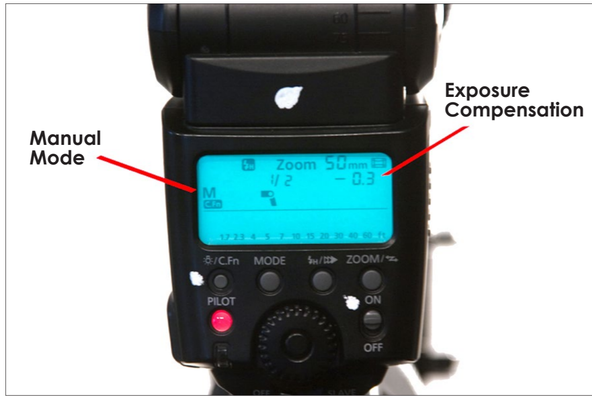
Figure 6. Set your strobe to manual control and adjust the exposure compensation.
