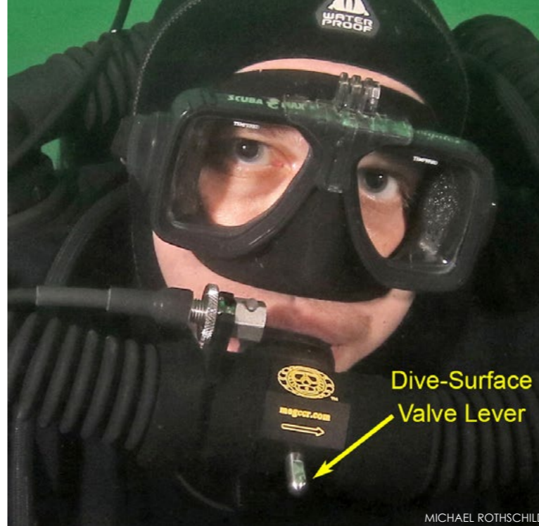
Figure 2: Dive-surface valve (DSV) vs. bailout valve (BOV)
