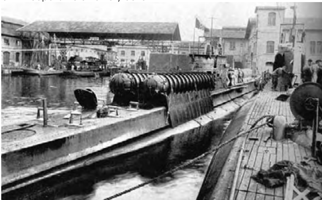
Italian Submarine Scire in the port of La Spezia with containers for two SLCs mounted on her deck
