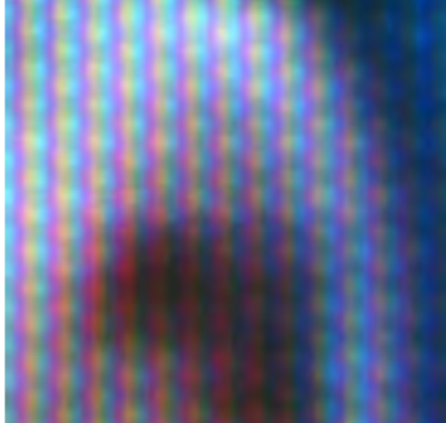
Figure 16. RGB colours revealed. This is a close-up photo of a computer monitor. See how every colour is blend of Red, Green and Blue pixels lighting up at various intensities (256 for each colour)
