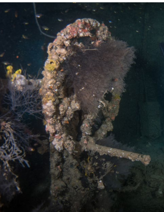
Manual ammunition lift to bring ammunition from below up to the gun on deck
