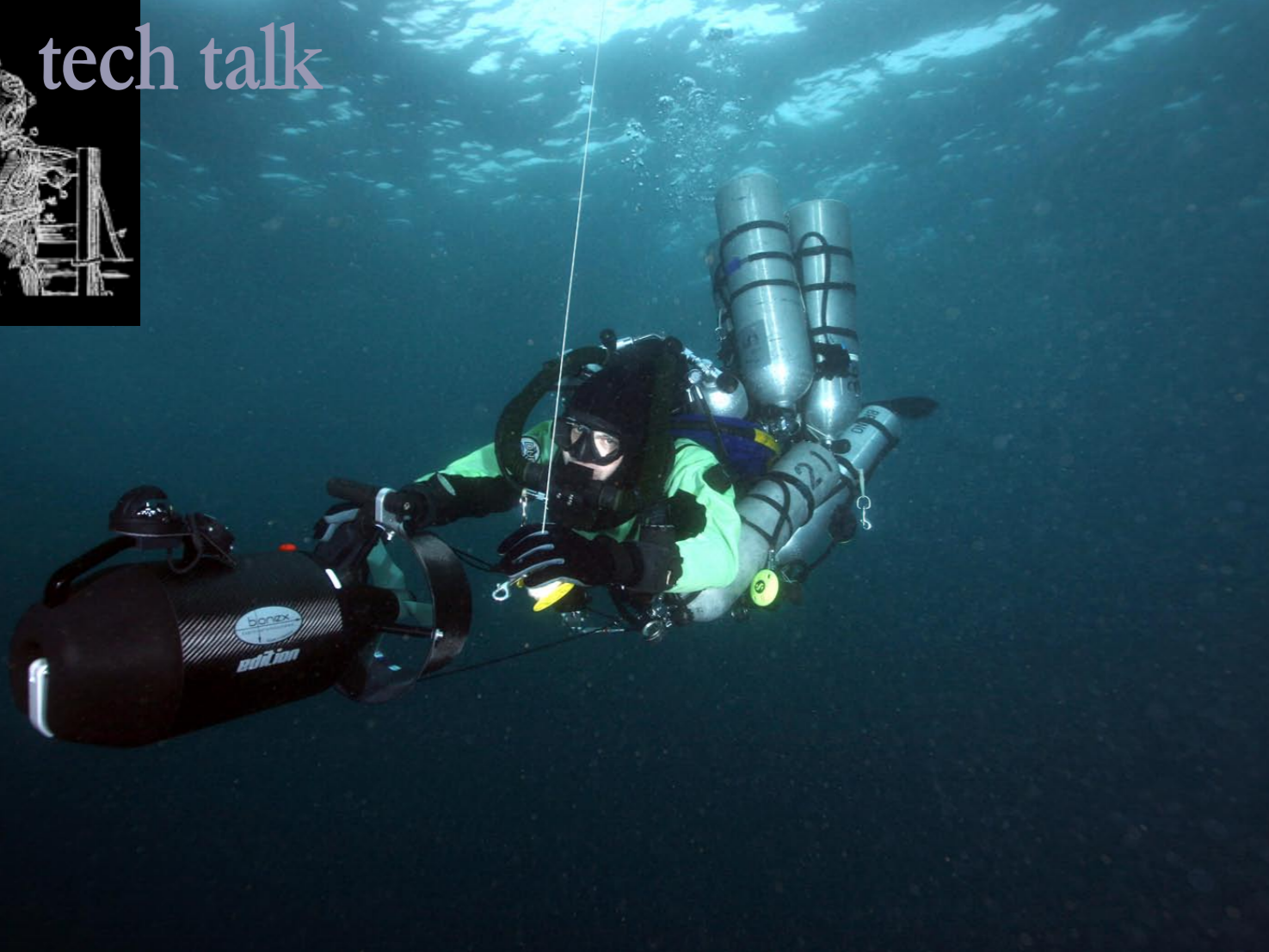
Technical diver on Semi-Closed Rebreather (SCR) with four stages and underwater scooter
