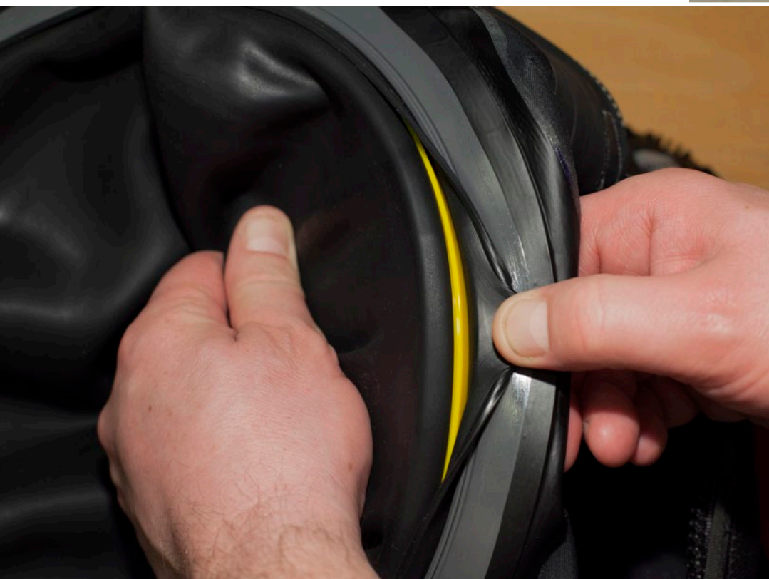
The yellow locking ring is visible above. This holds the neck cuff and is mounted at the edges, or with the included "pizza wheel" (top left).
